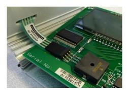
13) Place the spacers over the retaining screws on the front case.
