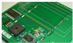
8) Locate the display orientation markers on the PCB and LCD.
