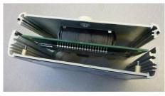
14) Remove the protective film from the LCD.
