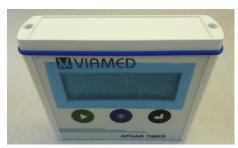
18) Insert the screw covers to all four screw holes.
