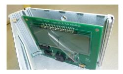
15) Guide the screws through the holes in the PCB then snap the two case halves together.
