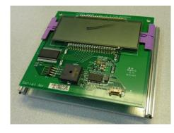
11) Solder the LCD to the PCB then remove the supports.
