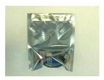
2) Take the sealed sensor and package it in a sensor box.
