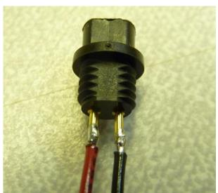
6) Cover the pins with the heat shrink. Shrink the tubing leaving none of the pin exposed.
