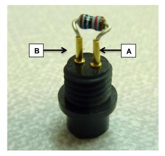
3) Solder the resistor in place. The resistor should lean slightly forward to allow the sensor wires to pass freely out of the connector hood.
