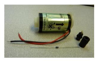
1) Take the  $10k\Omega$  resistor and shape the legs to fit into the connector pins.
