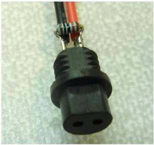
6) Screw the connector hood to the connector. If the resistor and wires are not compact enough then there may be resistance when tightening the hood, this can cause the pins to bend.
