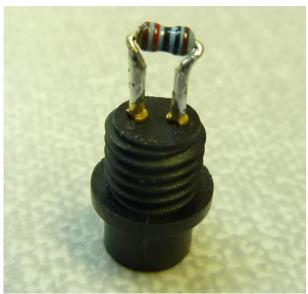
4) Place the connector hood over both sensor wires.
