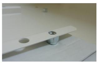
8) Place piece of folded card behind the nut to hold it in place.
