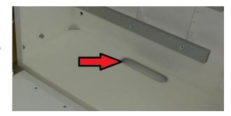
7) Inside the cabinet, on the rear panel, are three rail mounts. Place a nut behind the rail mount.
