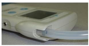
6) Connect the remaining end of the tubing to gas source with an inline flow meter.
