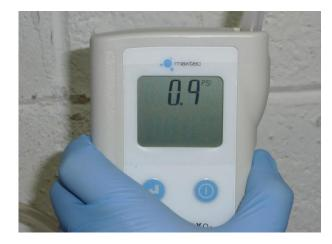
12) Set the pressure mode switch kPa. This can be found inside the battery compartment.
