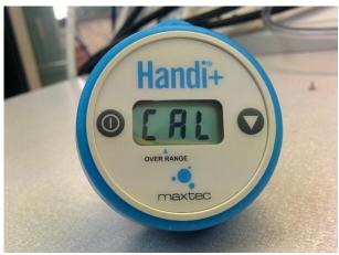
6) The analyser should display 20.9 when tested in air.
