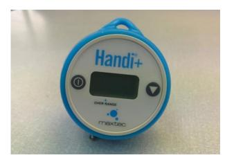
5) Press the **O** calibration button until CAL is displayed.
