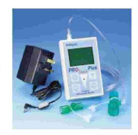
batteries and is supplied with mains charger/power supply. A sample-flow sensor enables the alarming of loss of sample.
