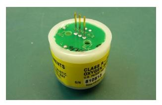
4) Noting the Red and Black marking on the sensor surface, place the PCB over the sensor's pin contacts as shown.
