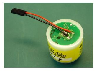
12) Using a low melt glue gun, cover the small PCB and its components in adhesive and allow to set.
