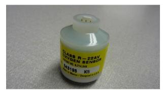
2) Remove the top cap from the sensor. Use VM3COP40.11 for the method.
