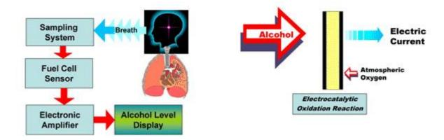
The Lion fuel cell has a high specificity to alcohols, and, although not totally ethanol-specific, it is very unlikely that the breath of a living human would ever contain any other chemical substance to which this sensor responds.
