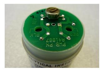
4) Using the flat edge of a Stanley knife, remove a small area of surface lacquer from in front of the solder contacts.
