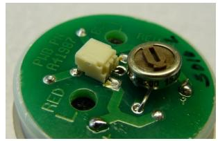
9) Solder the connector into place.
