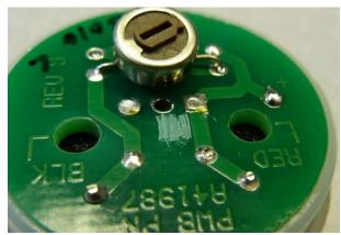
5) Using small pliers, remove the marked contacts.
