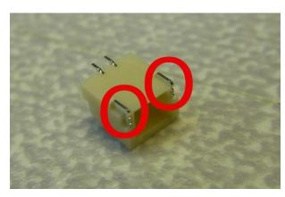
6) Splay the solder contacts to around a 30° angle.
