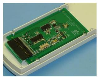
4. Solder the three control pot tabs to the contacts on the PCB.
