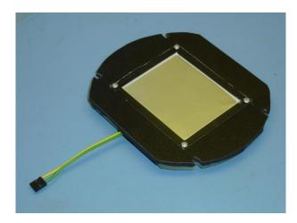
11. Using double sided tape, affix the transducer interface cushion to the inside surface of the upper case.
