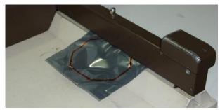
3. Fill the transducer cushion with water, leaving as little air in the cushion as possible, and seal.
