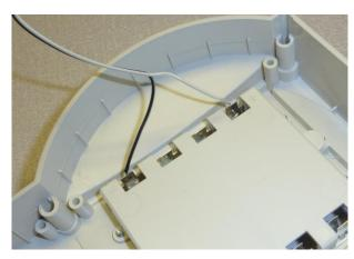
16. Connect the 2 pin M22 connector to the 2 pin connector on the PCB.
