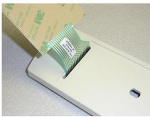
3. Remove the protective backing from the keypad to expose the adhesive backing.
