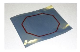
2. Seal the edges of the transducer cushion, leaving a small gap for filling.
