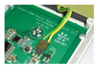
14. Cut a length of ribbon cable to 150mm. Affix a 2 pin M22 connector.
