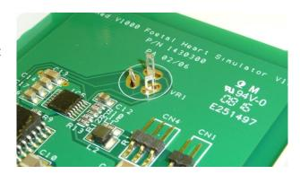
3. Using the PCB retaining screws, affix the PCB into place.
