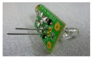
23) Solder the LED in place. The LED should be 7mm above the PCB.
