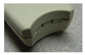
6) Mark a pilot hole for the strain relief.
