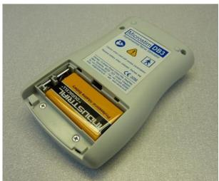
3. Without the patient lead connected, press and hold the P.T.C. button. If the battery is of sufficient Voltage, then the L.E.D. on the front of the Microstim will light up in green. If the L.E.D. lights in amber or red, then replace the test battery and repeat this step.
