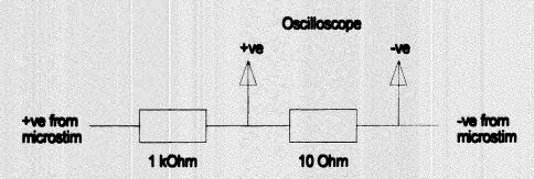
Typical pulse using this test adapter is shown below. This shape and amplitude of pulse is typical for all settings at maximum intensity. Pulse width is 200ms. Minimum setting on intensity pot should give zero output when scoped. Unit on which these results are based showed a slight jump in amplitude output with intensity pot increase, to 100mV from 0mV at approx 10% intensity.
