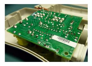
The quality of the soldering, while not first class, is sufficient. No serious faults were seen.
