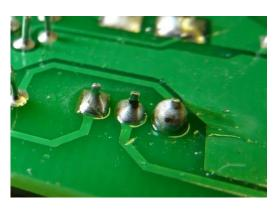
There were also a small number of more serious solder faults, such as the solder bridge shown here. These faults are likely to be related to the excessive component leg length.
