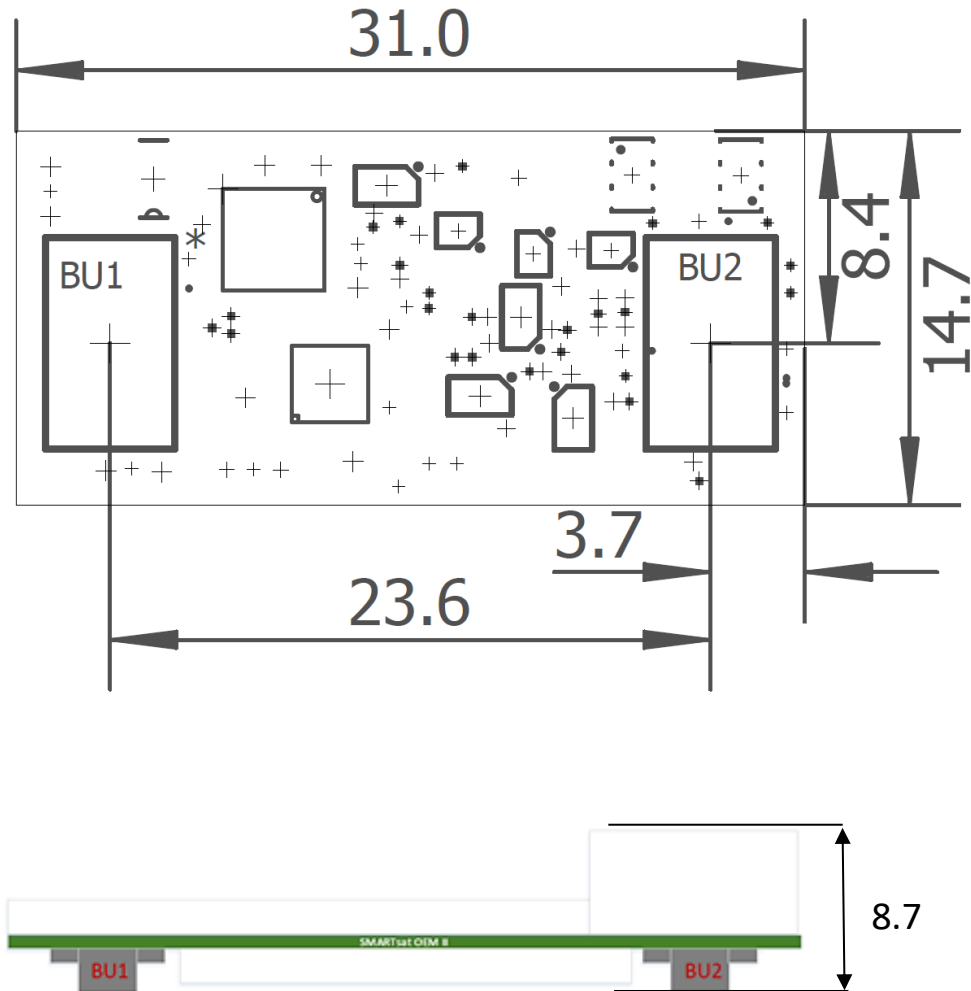
Fig. 3-3: SMARTsat® OEM II Board Physical Dimensions (in mm)
