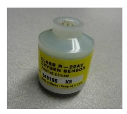
2) Remove the top cap from the sensor.
