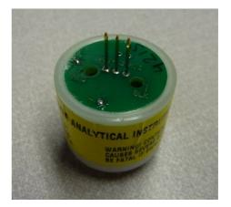
4) Using a soldering iron and pliers, remove the pins.
