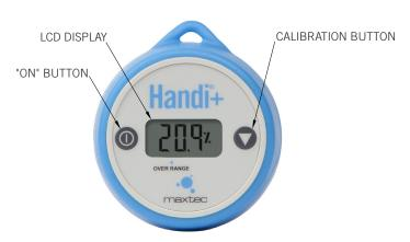
**LCD Display:** A 3-digit display provides a direct readout of oxygen concentration in the range of 0 - 100%. The display is blank when the Handi+enters its Sleep (power off) mode. The Handi+ will automatically enter the Sleep mode after approximately 1.3 minutes from the last time the ON button was pressed.
