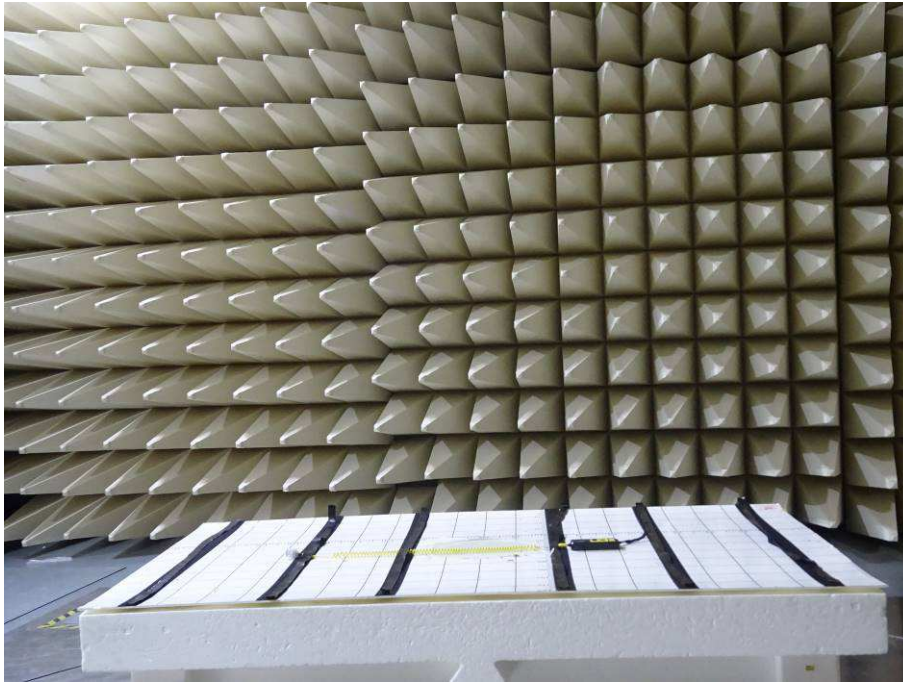
Fig. 1: Test set-up radiated emissions (tested together with VN202)
