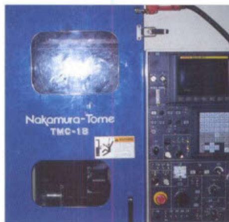
Effective design should incorporate easy-to-see and easy-to-use operating controls and emergency stop controls.
