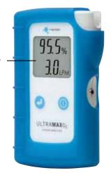
The UltraMaxO2 offers a fast and easy verification of oxygen concentration, flow and outlet pressure of oxygen concentrators
