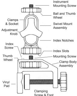
The Universal Mounting is used to attach instruments to IV poles, shelves and other objects up to 3.8cm thick. The Mounting Clamp offers 360-degree rotation and 180-degree movement in all directions providing maximum flexibility in selecting a mounting site.
