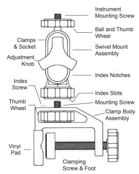
The Universal Mounting is used to attach instruments to IV poles, shelves and other objects up to 3.8cm thick. The Mounting Clamp offers 360-degree rotation and 180-degree movement in all directions providing maximum flexibility in selecting a mounting site.
