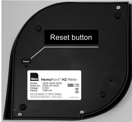
Illustration 35: Location of the reset button.
