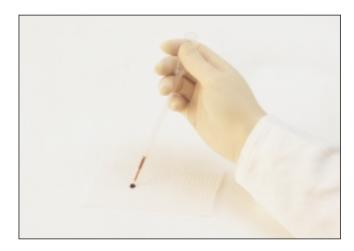
Introduce the cuvette into the middle of the drop in such a way that the cuvette is filled in one step. It should never be topped up.
