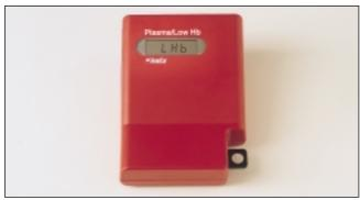
The letters "LHb" should now be seen on the display. If not, check the connections to the photometer and to the main power supply. If the photometer is still not functioning after these checks, turn to "Troubleshooting Guide," page 16.
