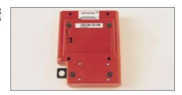
Place five batteries, type R6 or AA, in the battery compartment observing the indication of polarity in the battery holder. Replace the lid. New batteries can operate continuously for approximately 100—150 hours. If battery powered, batteries can be readily conserved by switching off the photometer between measurements.
