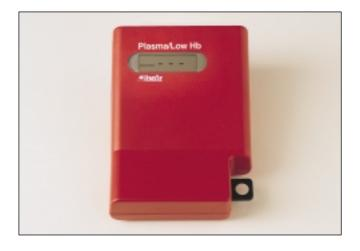
In less than one minute the photometer displays the result. Compare this value to the assigned value on the Plasma/Low Hb Control solution vial. If the result is out of range refer to "Troubleshooting Guide", page 16.
