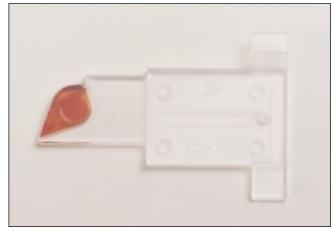
Place the filled cuvette into the cuvette holder and carefully push it into the measuring position. The filled cuvette should be analyzed immediately and at the latest within 1 minute after filling. Filled cuvettes are to be kept lying down.
