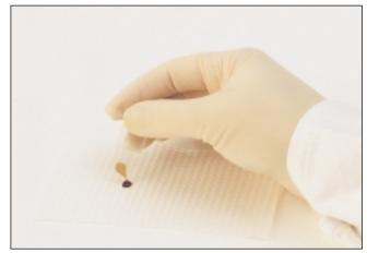
Using laboratory tissue, carefully wipe off the excess sample on the outside of the cuvette. Make sure that no sample is drawn out of the cuvette during this procedure.
