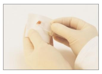
The filled cuvette should be visually inspected to check that the cuvette is properly filled i.e. completely filled up to the edge and without air bubbles in the optical eye.
