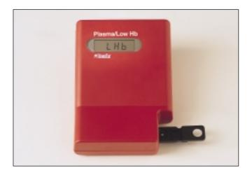
After approximately 15 seconds the indication "READY" appears on the display together with three flashing dashes. The photometer is ready for measurement.
