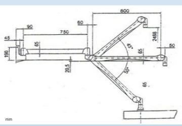
0310305 With double-jointed wall mounting & with height adjustment
