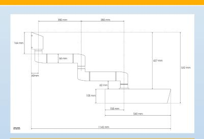
With double hinged arm & wall mount bracket, with integrated electrics
