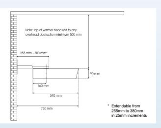
With fixed wall mounting bracket, not pivotal
