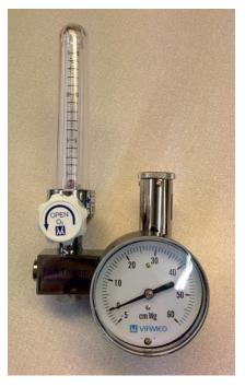
2) Set the adjustable valve to minimum (fully counter clockwise).
