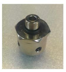
Unscrew the adjustable valve from the right hand threaded hole on the top face of the body block.
