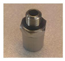
7) Unscrew and remove the precision valve.
