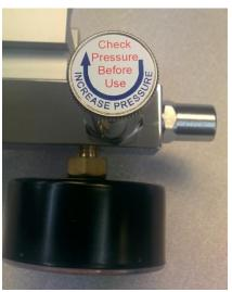
3) Connect the inlet to the oxygen supply at a pressure of 4 bar.
