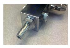
4) Ensure the port and threads are free of foreign matter. Replace the thin O-ring (P/N 0330214).
