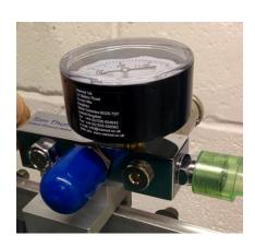
9) Slightly unscrew the adjustable valve and apply oxygen compatible adhesive to the exposed threads. Retighten the adjustable valve with the 7/8 A/F spanner.
