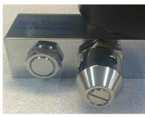
8) See valve servicing manual to service this valve. Ensure the port and threads are free of foreign matter. Remove the thin O-ring and replace with a new O-ring (P/N 0330214).
