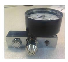
2) Ensure the port and threads are free of foreign matter. Replace the thin O-ring (P/N 0330214).
