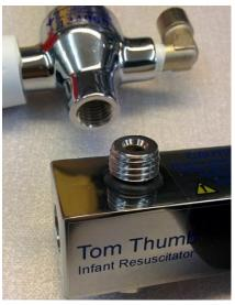
12) Ensure the port and threads are free of foreign matter. Replace the thin O-ring (P/N 0330214) with the thick O-ring (P/N 0330213).
