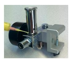
10) Check for TT pressure gauge sticking. Release and cover the T piece adapter port a number of times, ensuring that TT pressure gauge returns to 45±1 cmH2O. Uncover the precision valve holes.
