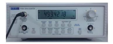
Example shows reading at 120 bpm, i.e. target value 500.00 ms. Displayed measured reading to record = 499.42 ms.
