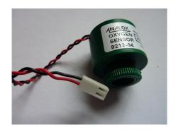
Electrical connections. 10.5mV in Air Red is =+ve Black is -ve
