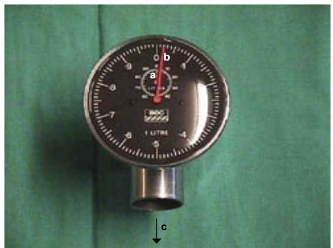
3 Wright's respirometer. a Small pointer shows accumulated volume; b large pointer indicates tidal volume (it can be reset each breath); c to the breathing system.
