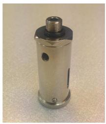
12) Screw the adjustable valve into the remaining threaded hole in the bottom face of the body block. Use the 7/8 AF spanner to tighten.
