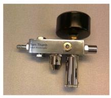
19) Attach the spacer block to the body block using 2x M4x10mm hex drive bolts. Use a 3mm Allen key to tighten.
