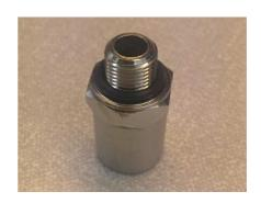
18) Screw the 15mm outlet into the threaded hole in the right face of the body block. Use 5/8 AF spanner to tighten
