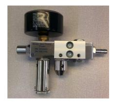
20) Attach rail clamp to the spacer block using 2x M4x10mm hex drive bolts. Use a 3mm Allen key to tighten.
