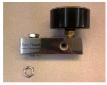
8) Screw the flowmeter blocking bolt nut into position. Use 2x 5/8 spanner to tighten.
