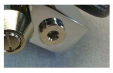
16) Place a thin O ring over the thread of the adjustable valve.
