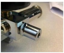
20) Attach the spacer block to the body block using 2x M4x10mm hex drive bolts. Use a 3mm Allen key to tighten.
