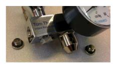
13) Place a thin O ring over the thread of a blanking bolts.
