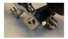
15) Screw into the right hand threaded hole on the bottom face of the body block. Use a 5mm Allen key to tighten.
