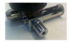
19) Attach the spacer block to the body block using 2x M4x10mm hex drive bolts. Use a 3mm Allen key to tighten.
