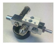
20) Attach rail clamp to the spacer block using 2x M4x10mm hex drive bolts. Use a 3mm Allen key to tighten.
