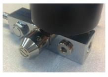
17) Place a thin O ring over the threaded end of the 15mm outlet
