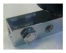
9) Place a thin O ring over the thread of the adjustable valve.
