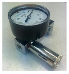
11) Place a thin O ring over the thread of the precision valve.
