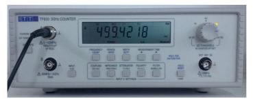
Example shows reading at 120 bpm, i.e. target value 500.00 ms. Displayed measured reading to record = 499.42 ms.
