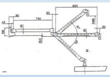
With double-jointed wall mounting & with height adjustment Model: 521A-60025-3-EX
