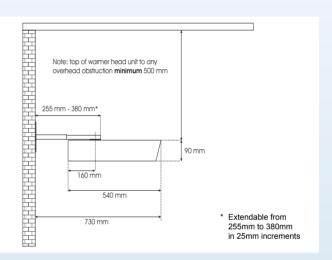
With fixed wall mounting bracket, not pivotal
