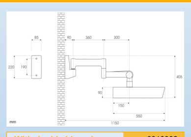
With double hinged arm & wall mount bracket, with integrated electrics
