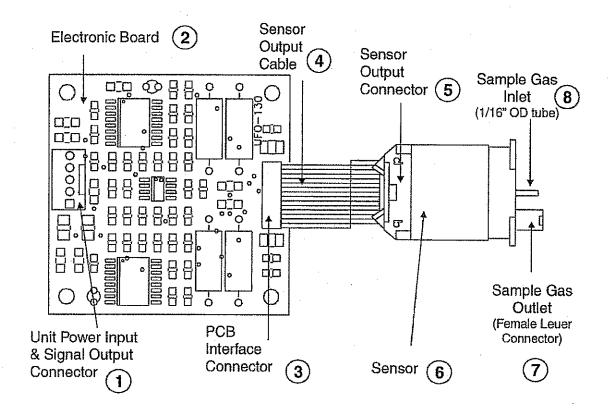
Fig. 1 Sensor - PCB Assembly Top View
