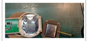
Peel off the old transducer interface cushion. Replace the double sided tape if necessary. Affix a new transducer interface cushion in the space between the support posts.
