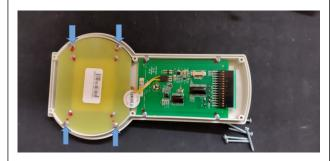
Remove the transducer assembly. Note the position of the four M4 nuts used as spacers under the transducer assembly.
