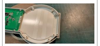
Carefully place the transducer assembly on the four M4 nut spacers and hold in place with the four screws and washers.
