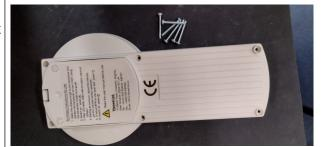
Split the two halves. Take care, the power lead will be connected between the halves.
