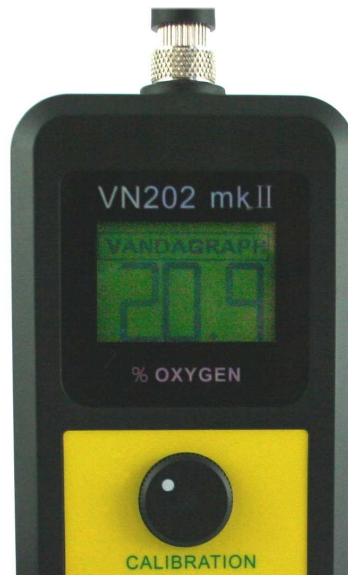
Fig.6 – Analyser display after calibration
