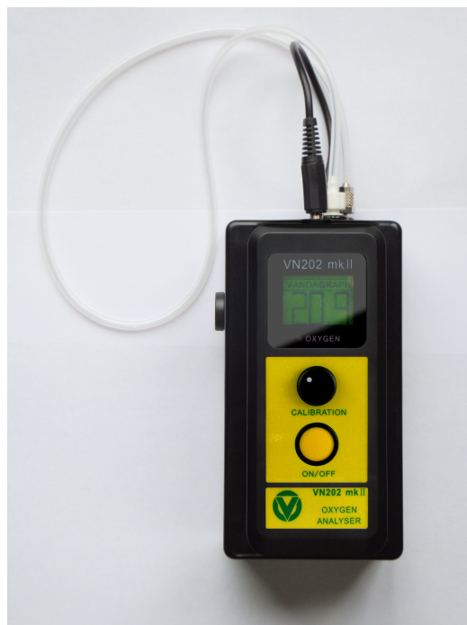
Fig.1 – VN202 mkII Oxygen Analyser with Gas Analyser Pump Box
