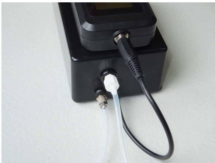
Fig.4 – Connecting the pump box to the analyser
