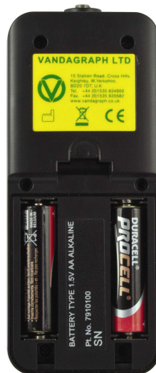
Fig.2 – Battery location in the VN202 mkII Oxygen Analyser
