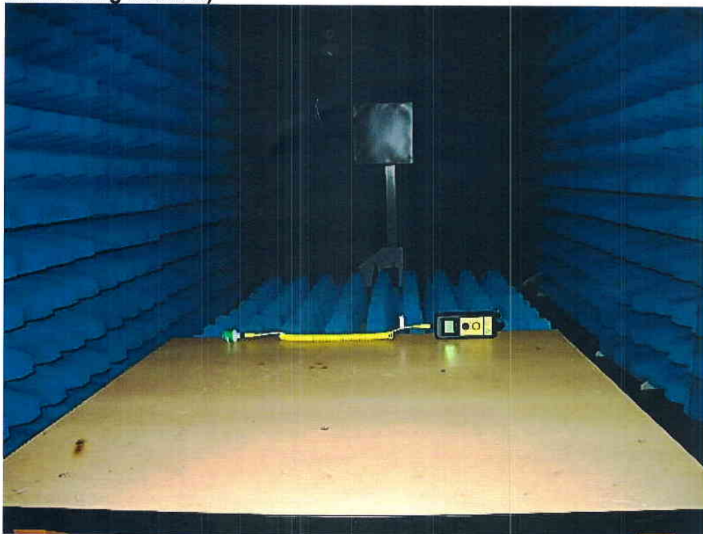
Photo 6 Radio Frequency Electromagnetic Fields Immunity test (with connecting cable A)
