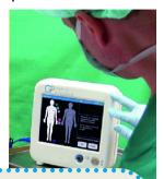
The monitoring system measures patient's skin surface temperatures at 6 defined dermatomes using **non-invasive sensors** and displays the levels of anaesthetisation. It helps physicians to react quickly for adverse effects like Total Spinal Anaesthesia (TSPA) or Apnea.
