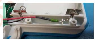
INSERT Battery cable contacts into enclosure.
