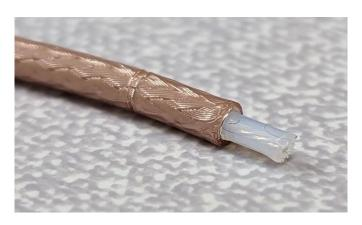
6) Remove the clear plastic cable inner, as shown. Ensure that there are no excess strands of the outer shield near the wire core.
