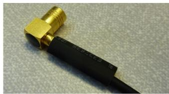
31) Using a heat gun, shrink the heat shrink into place. Ensure that the heat shrink is flush to the connector body.
