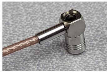
15) Place the crimp into the large hole of the crimp tool, ensuring the crimp is still flush to the connector body.
