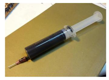
25) Fill the connectors with the resin. Try to avoid leaving air gaps.
