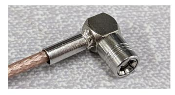
14) Using the pick, tuck any excess shield into the crimp. Push the crimp up to the connector body. The crimp must be flush to the connector body with no strands of shield showing.
