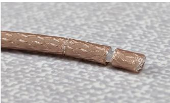
5) Remove the outer cable sheath and braided shield.
