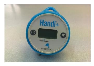
2) Press the calibration button until CAL is displayed.
