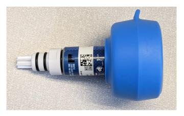
5) Connect the gas sample tubing to the calibration assembly and the UN1072 Oxygen source.
