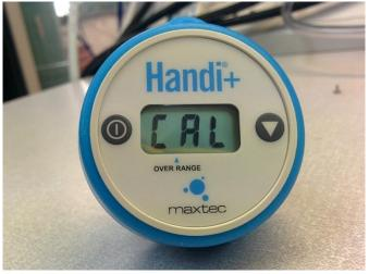
3) The analyser should display 20.9 when tested in air.
