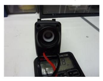
2. Switch on using the mA range ( The uA offers too high an impedance The reading should be less than 5mA and the LCD should show a reading
