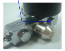
5. Unscrew the 10mm inlet from the left hand face of the body block. Ensure the port, and threads, are free of foreign matter. Replace the thin O-ring (p/n 0330214) and refit the 10mm inlet.
