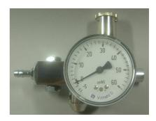
9. IF pressure gauge can be removed without spanner, OR pressure gauge is not straight.
