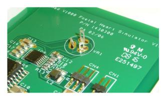
3. Using the PCB retaining screws, affix the PCB into place.
