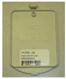
23. Affix a trimmed serial number label to the inside of the battery compartment.
