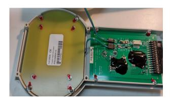
22. Affix a serial number label to the inside of the battery compartment door.
