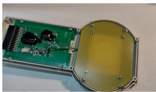
13. Connect the transducer assembly to the PCB using the 3 pin connector.
