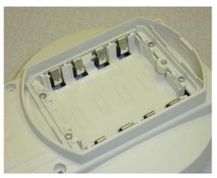
6. Place the battery compartment seal into the channel around the perimeter of the battery compartment and push into place.
