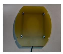
10. Place the transducer surround on the transducer mounting board.
