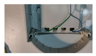
16. Connect the 2 pin M22 connector to the 2 pin connector on the PCB.
