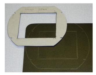
We now have a laser cut part. V1000 Transducer Interface Gasket 1430299
