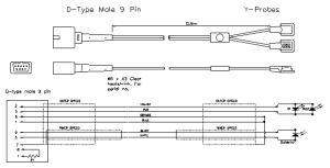
R1 - 7.5 K DHW 1%, 1/8W RESISTOR \* INNER SHIELD AND OUTER SHELD TO BE TANSTED TODETHER
