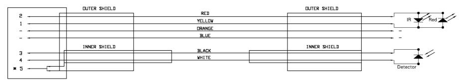
\* INNER SHIELD AND DUTER SHIELD TO BE TWISTED TOGETHER.
