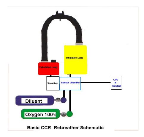
The actual location of various components will vary from manufacturer to manufacturer however the end result should be the same. The Diluent and Oxygen can be fed into the system at other points. This diagram is just one example. The objective is to re-cycle the oxygen by removing  $CO_2$  and replacing the Oxygen used and converted into  $CO_2$  with fresh Oxygen.
